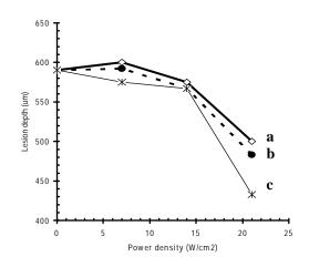
**Fig. (1):** The relation between the lesion depth and the power density in continuous group. Exposure time was (a) 0.3 s (b) 1 s and (c) 3 s.
